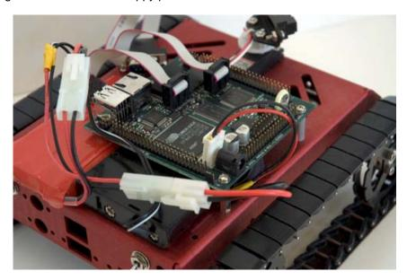
**Warning**: you can only power the iPac-9302 via the banana plug or floppy power connector, but not at the same time. Applying power to both power sockets could result in injury and damage to the board.
